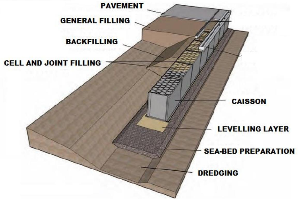
**Construction approach for docks and breakwaters using caisson-type solutions**
