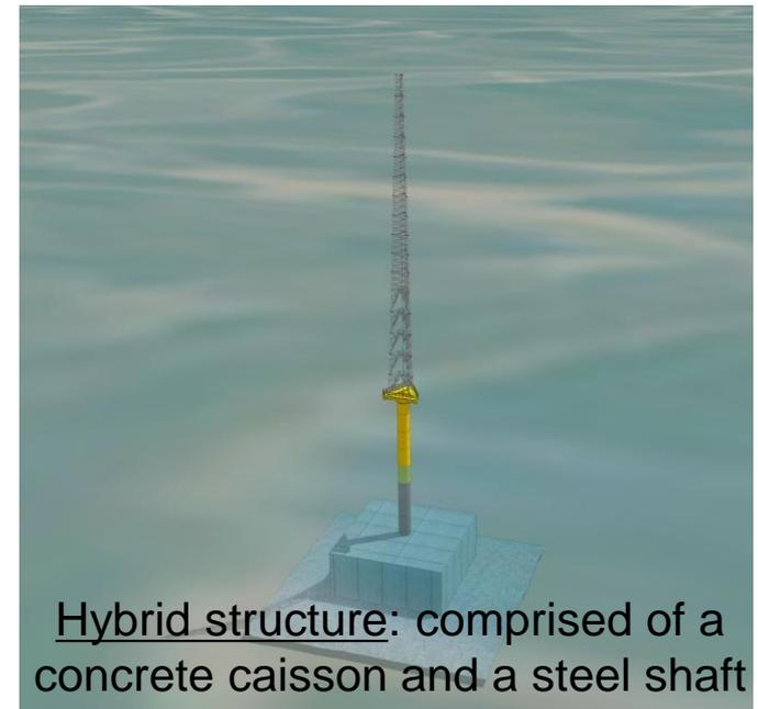
Hybrid structure: comprised of a concrete caisson and a steel shaft
