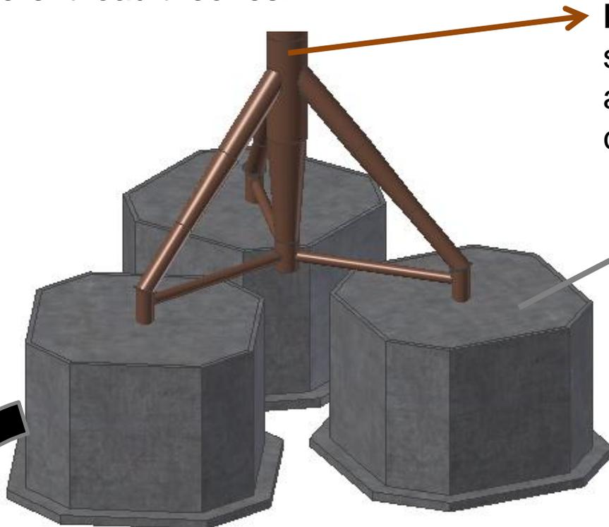
**Morison's equation:** Wave loading on slender elements associated to the inertial and draft forces (mass and drag coefficients needed)
